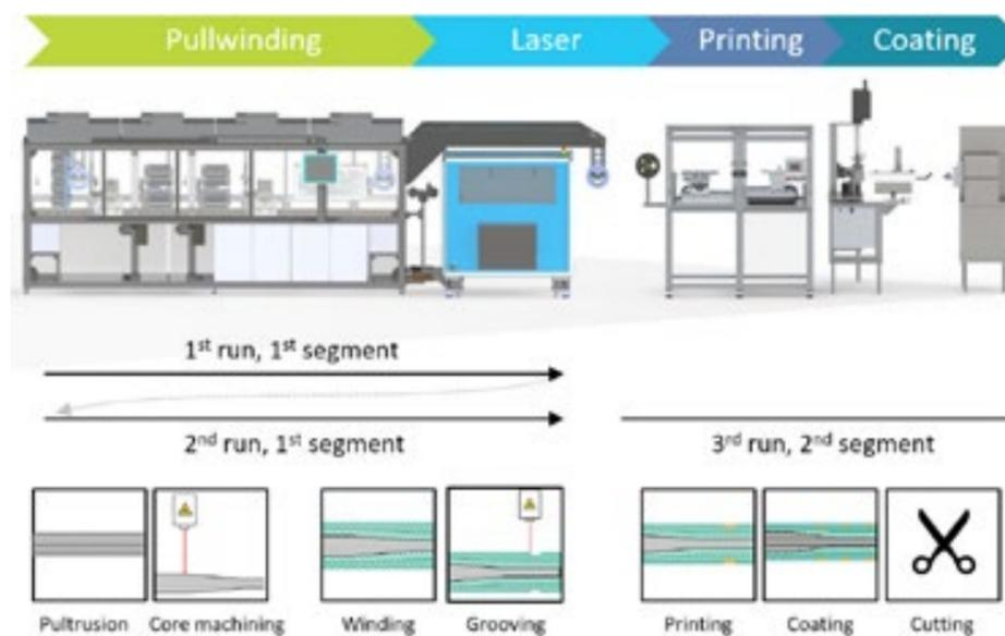
Figure 1: Concept of OPENMIND process
