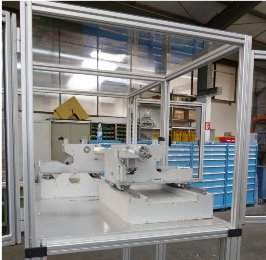
**Figure 8: Print head – mounted on movement unit**
