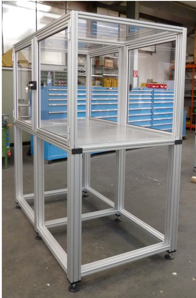
Figure 1: Machine pedestal – assembly of frame with doors and base plate
